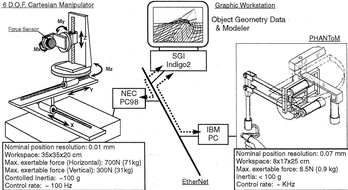
**Fig. 1 ViSurf System Configuration** The system has 2 force feedback devices which asynchronously communicate with a graphic workstation over the EtherNet (dotted lines with arrows). Haptic rendering on each PC is done based on shape features sent by the modeler on the workstation.
