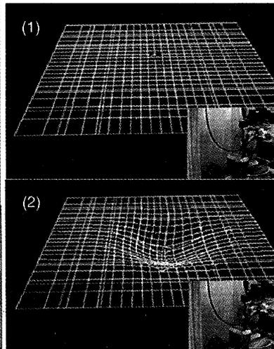
**Figure 2. Deformation with curving tool; LEFT: polygonal surface, RIGHT: B-Spline surface**
