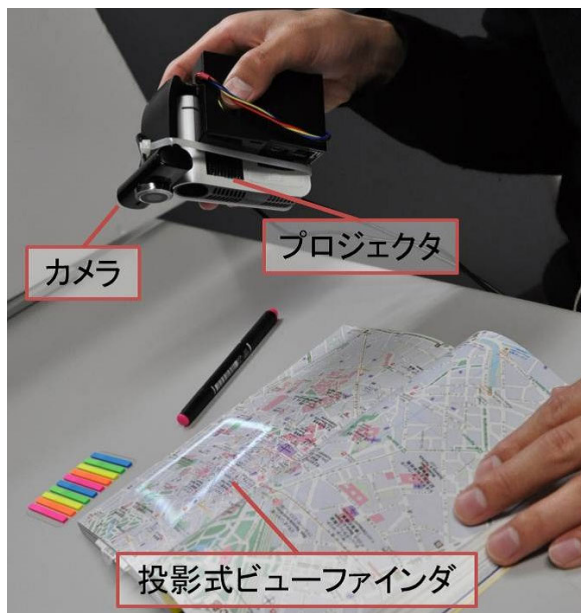
図 1 ClippingLight 使用例 Fig. 1 A user is wielding ClippingLight to clip part of image in the book
