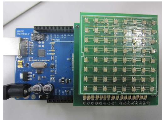
**Fig. 5** Developed bi-color dot-matrix LED unit and ArduinoMega controller.
