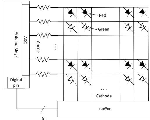
**Fig. 4** Circuit configuration of Bi-color LED Tile (bLT) device.
