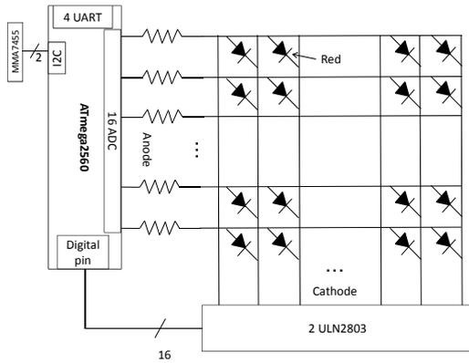
**Fig. 2** Overview of extended LED Tile (eLT) device
