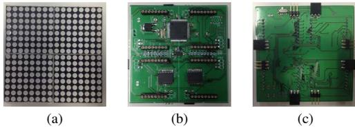
**Fig. 3** Developed eLT device. (a)front side, (b)front side under LEDs, and (c)back side.
