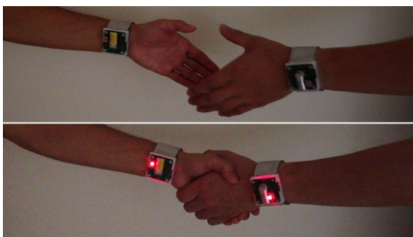
図 4 握手の検知 (LED による報知) Figure 4 Detecting shake hands represented by LED indicators
