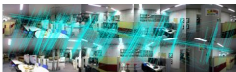
(a) Feature point matching by using RANSAC.
