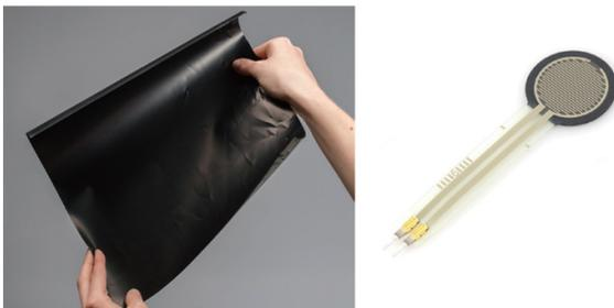
図 4 Velostat(Pressure-Sensitive Sheet)・FSR(Force-Sensing Register) Sensor
