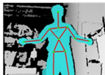
図 8 Kinect 処理の様子 Figure 8 Skeleton extraction from depth image
