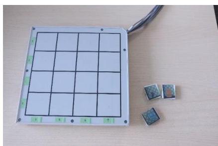
Figure1 Drawings of matrix RFID reader.
