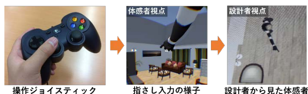
図 3 体感者から設計者への指さしによる意思表示 Figure 3 Occupant can point to objects in VR environment by tilting a joystick.
