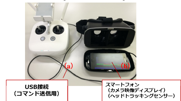
図3 HMD構成 Figure 3 HMD Configuration.
